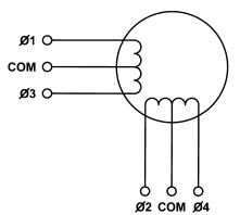
Figure 3: Step Motor Phases
